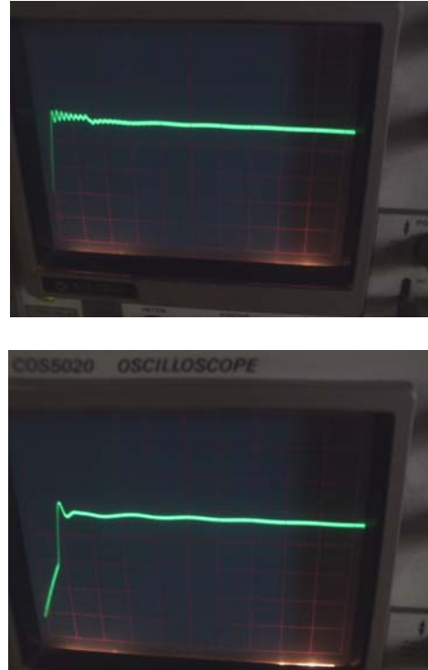
Fig. 3 PWM signal before (top) and after a compensator is added (bottom)
